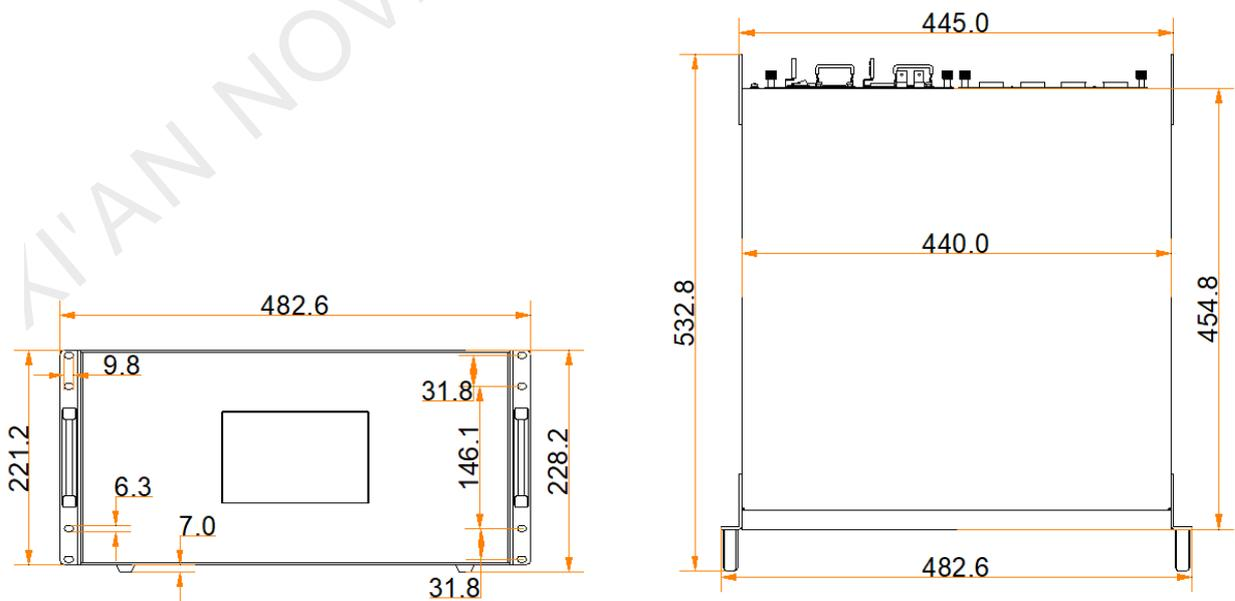
Tolerance:  $\pm 0.5$  Unit: mm
